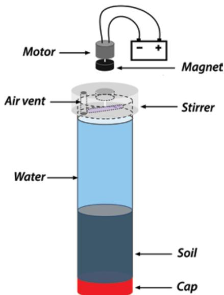
Figure 6.2: Experimental set up used to simulate soil flooding.
