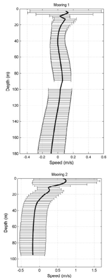
Figure 2.3. Mean currents (solid line) and variations in current (horizontal lines) on either side of the sill at the Rigolet Narrows. The variation is shown as a single standard deviation.
