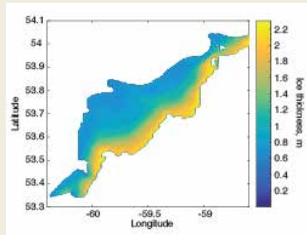
Figure 2.7. Model simulation of monthly mean ice thickness (m) in Lake Melville for February.
