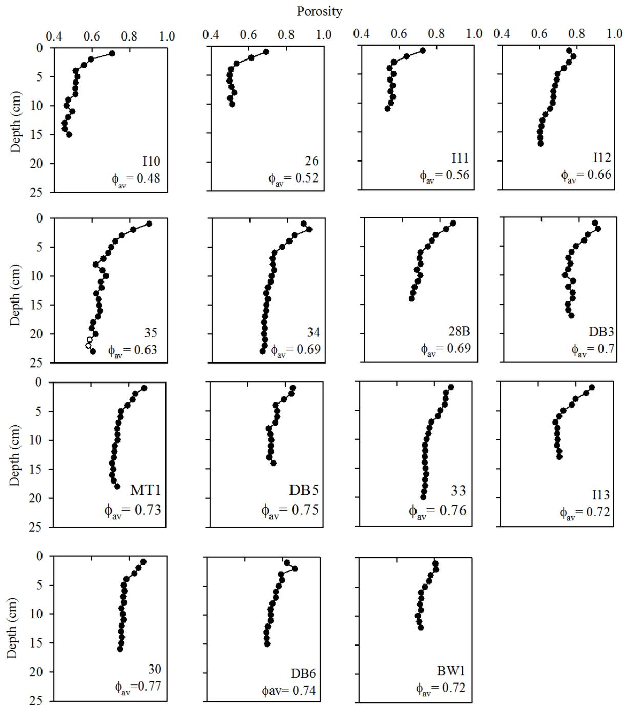
Figure 10.1. Porosity profiles of sediment cores. Values for average porosity ( $\phi_{av}$ ) are provided for each core. Core name is shown in the bottom right corner of each plot.
