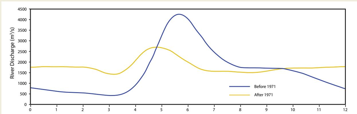
Figure 2.5. Variations in river discharge from the Churchill River due to the impact of the Upper Churchill hydroelectric facilities built in 1971. The figure shows the monthly mean Churchill River discharge calculated for two periods of time: before (blue curve) and after (yellow curve) 1971.
