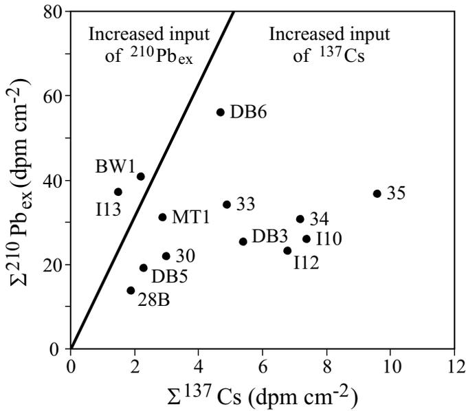
Figure 5.7. Excess  $^{210}\text{Pb}$  ( $^{210}\text{Pb}_{\text{ex}}$ ) and  $^{137}\text{Cs}$  inventories and their ratios in sediment cores compared to the expected inventories from direct atmospheric fallout (straight line).
