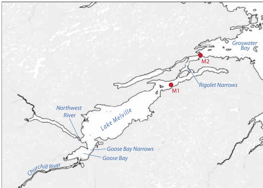
Figure 2.1. Locations of the two current meter moorings (M1 and M2) relative to the sill at the Rigolet Narrows. Source: Adapted from Lu et al. (2013).
