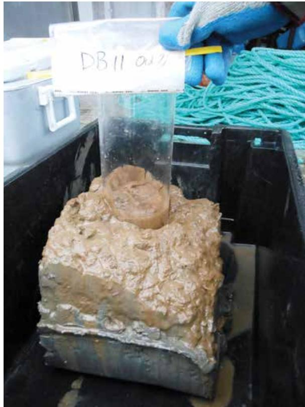
Figure 5.2. Sub-sampling of retrieved sediment using a push tube.
