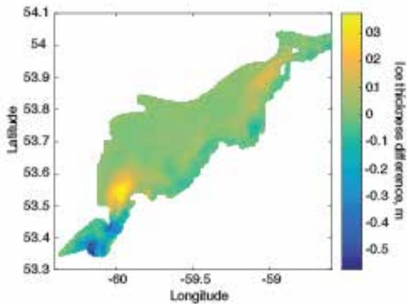
Figure 2.12. Differences in ice thickness (m) in February in the two model experiments calculated with river discharge after 1971 minus salinity in the model experiment with river discharge before 1971.
