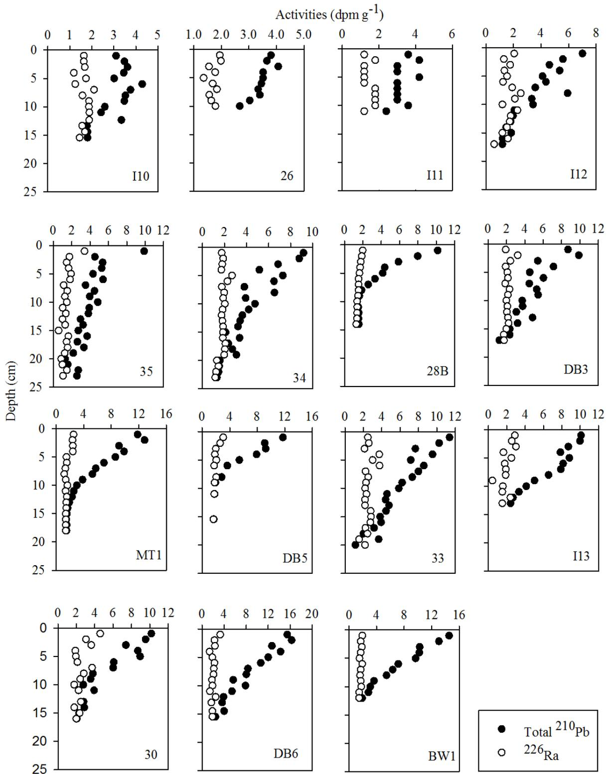
Figure 10.2. Profiles of total  $^{210}\text{Pb}$  (black dot) and  $^{226}\text{Ra}$  (white dot) activities in the cores. Core name is shown in the bottom right corner of each plot.
