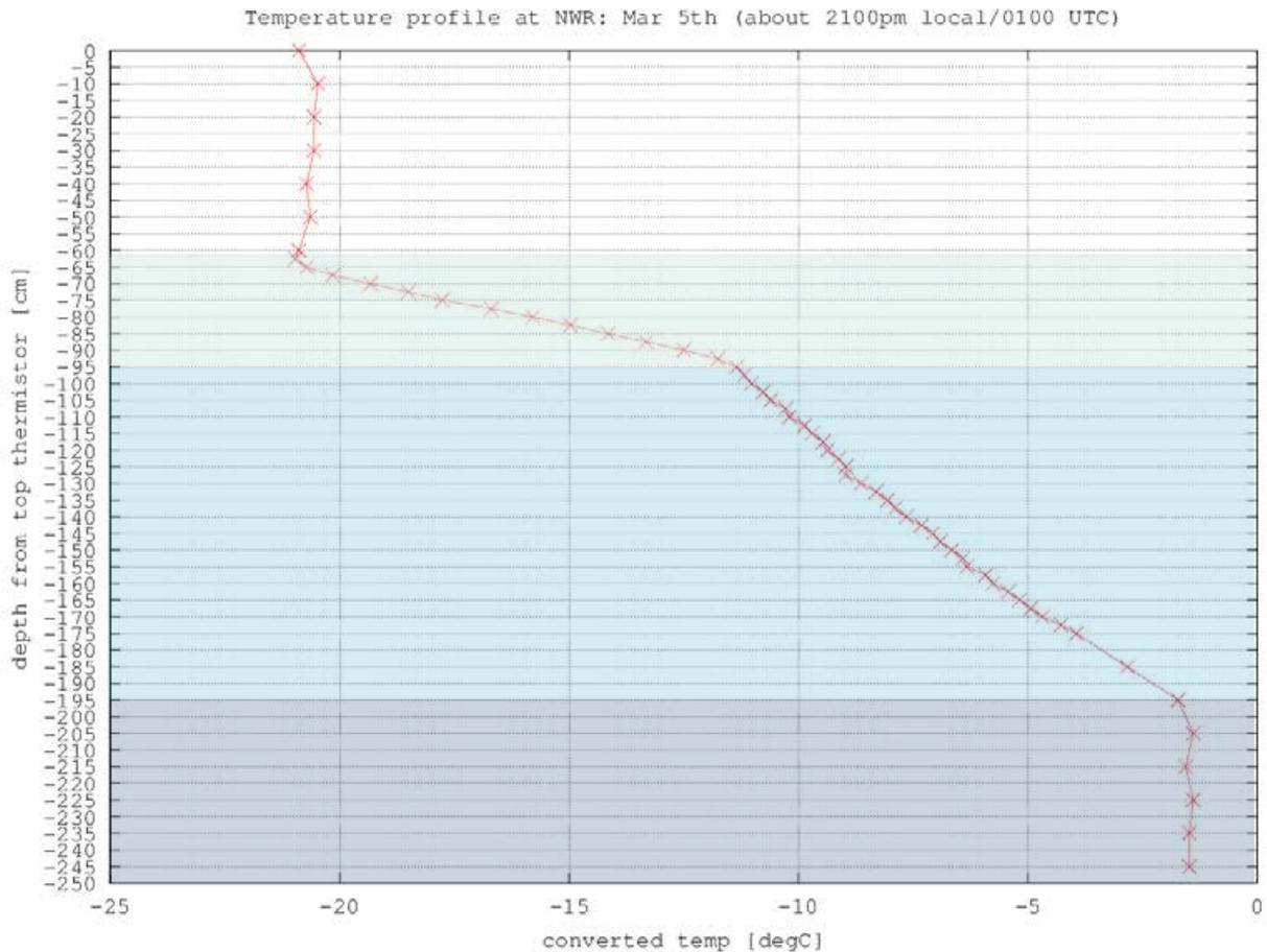
Figure 4.5. Temperature profile for the air (white), snow (green), ice (blue) and water (grey) at the North West River SmartSENSOR on March 5<sup>th</sup>, 2015. Using the temperature profile, the depth of snow (~30 cm) and thickness of the ice (~100 cm) can be inferred.
