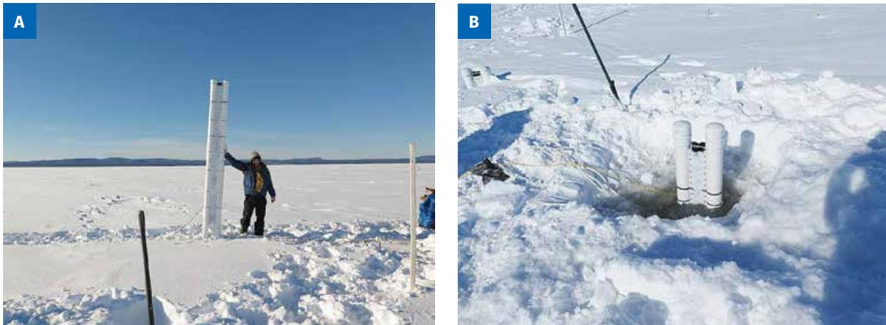
Figure 4.4. Photographs showing (a) the complete North West River SmartSENSOR with a researcher shown for scale and (b) the installation of the prototype through the ice near North West River.
