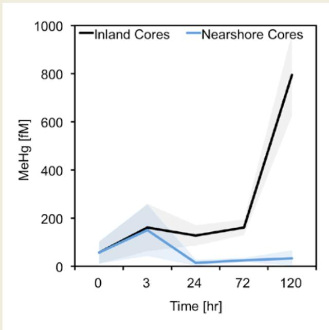
Figure 6.11. Changes in methylmercury (MeHg) concentrations over time in overlying water of experimentally flooded soils from the Lake Melville watershed. Results are from six cores from the planned reservoir area. Three were collected near the Churchill River and three from the dry inland regions that will be flooded. Source: Schartup et al. (2015).
