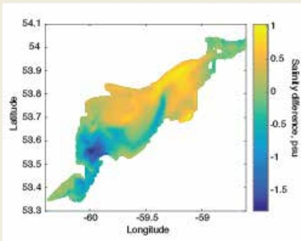
Figure 2.9. Winter season: Differences in salinity (psu) in the two model experiments calculated with river discharge after 1971 minus salinity in the model experiment with river discharge before 1971.
