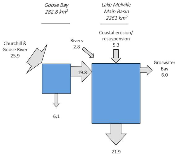
Figure 5.3. Mass balance budgets of sediment ( $\times 10^8 \text{ kg yr}^{-1}$ ). Arrows pointing towards a box represent inputs and arrows pointing downwards represent sinks.
