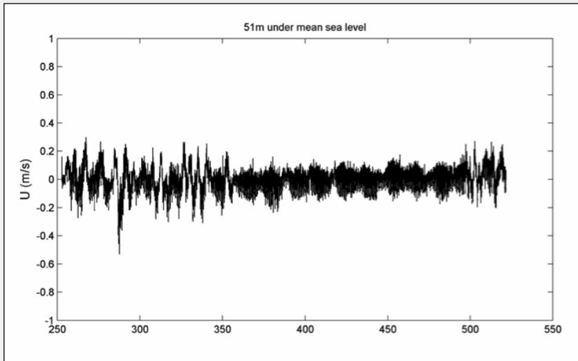
Figure 2.4. Currents from September 2012 to June 2013 in Year Days (counted from 1 January 2012) at 51 m depth at M1 inside the sill in Lake Melville. The U component represents the horizontal velocity with direction along the axis of the lake (i.e. movement in and out of the lake). The drop in currents from December 2012 (around day 350) to late April 2013 (day 500) is because of the formation of ice.
