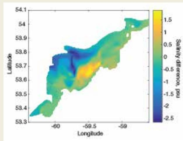
Figure 2.10. Summer season: Differences in salinity (psu) in the two model experiments calculated with river discharge after 1971 minus salinity in the model experiment with river discharge before 1971.
